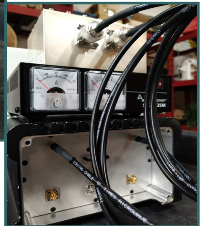
Rear View w/ Power Supply and Duplexer. Note that the RF cables are cut very long for the prototype. Final version will be cut to length. Also note that the internal Duplexer is not connected.
